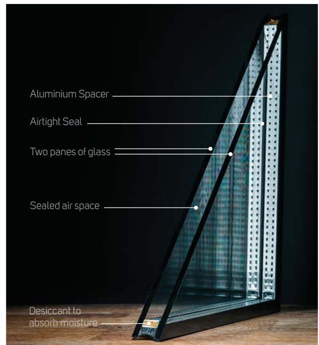
Above: The components of an Insulated Glass Unit (double glazed).
